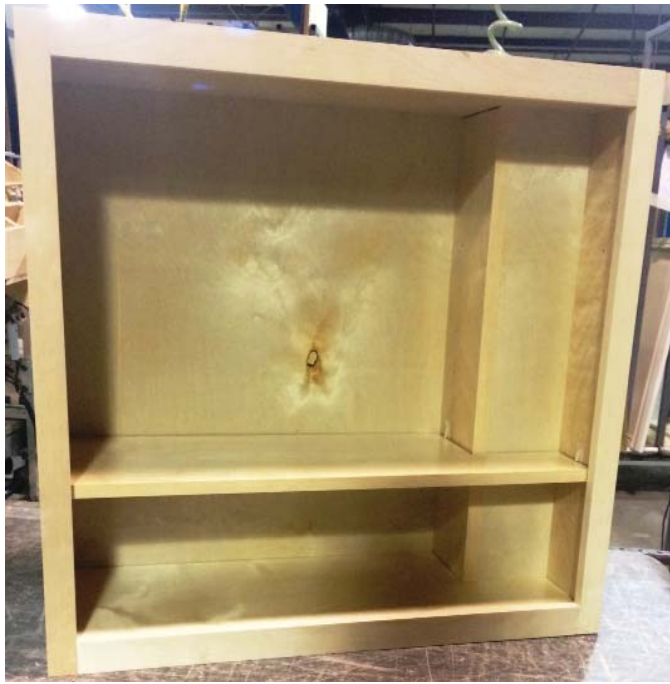
Pipe chase on the right end of the cabinet.
